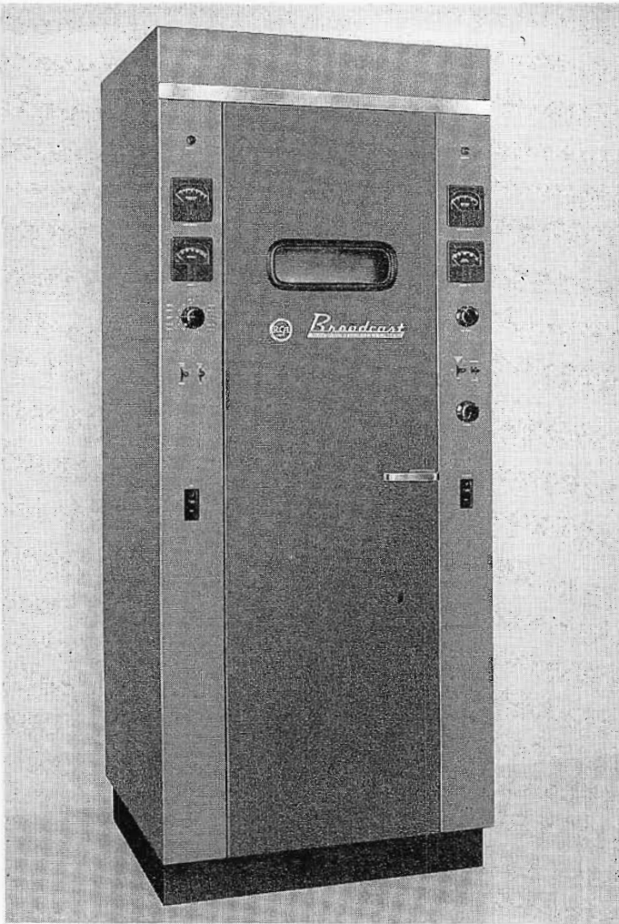
FIG. 6. The BTA-1R 1000 watt AM transmitter used by WONA. An adjoining rack contains input equipment. This type installation is ideal for stations planning to operate by remote control.
