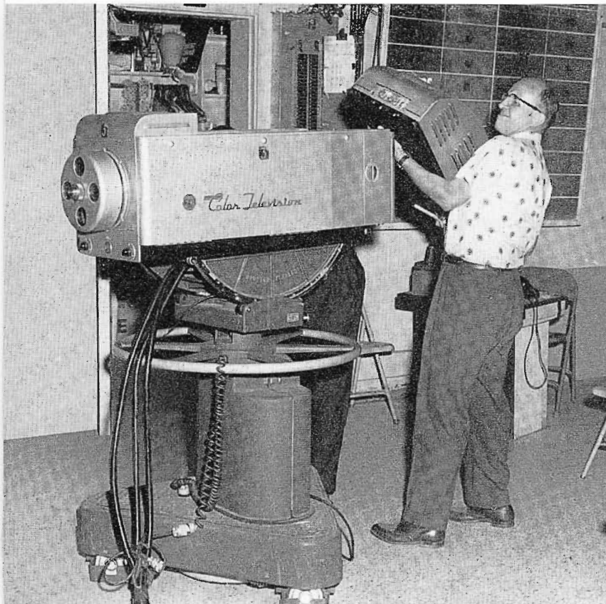
FIG. 8. As soon as the day's studio color schedule is completed, engineers make color equipment ready for baseball telecasts. Here a color camera is dismantled prior to moving it to the mobile unit.
