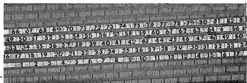
FIG. 1. Close-up of headwheel panel of the RCA TV Tape Recorder showing how video heads apply transverse tracks on tape. Tracks shown here are an artists conception of video information applied to tape. Extreme close-up below shows detail of tracks—note that each scanning track is made up of 18.4 horizontal TV lines.
